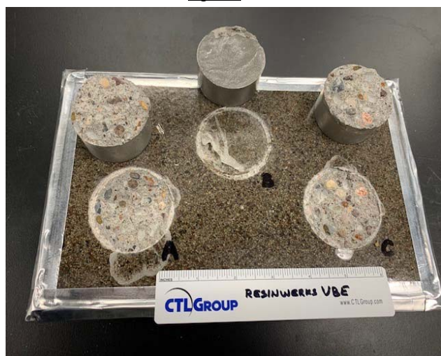
Figure B Pull results on Resinwerks VBE @ 12 mils.
